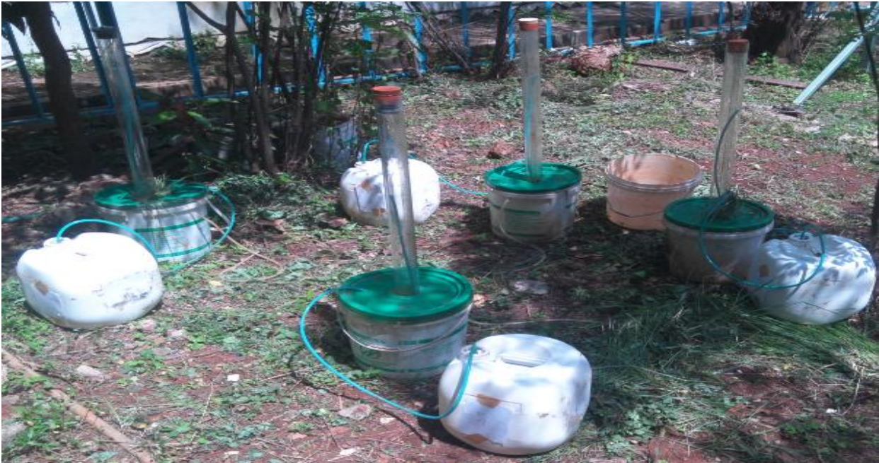
Figure 3.2: Experimental setup of anaerobic co-digestion for initial pH effect determination
