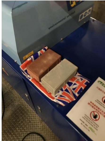
Figure 3: Cullet-clay Bricks Produced from Recycling Glass Bottles
